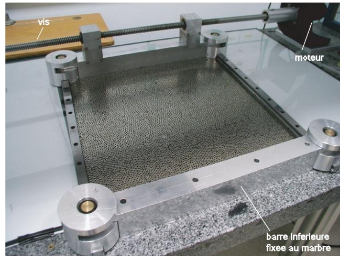
Figure 3: A bi-dimensional, bi-disperse granular material, composed of about 8.000 metallic cylinders of diameter 5 and 6 mm in equal proportions, is sheared quasi-statically in an horizontal deformable parallelogram. The shear is periodic, with an amplitude \theta_{max} = \pm 5^\circ . The volume fraction ( \phi = 0.84 ) is maintained constant by imposing the height of the parallelogram. The dynamics of 2818 grains located in the center of the device is followed by a High Resolution Digital Camera which takes a picture each time the system is back to its initial position \theta = 0 . The microscopic unit of time is one cycle, a whole experiment lasting 10.000 cycles. Experiments with this setting have been performed and analyzed in publications by Dauchot et al.
